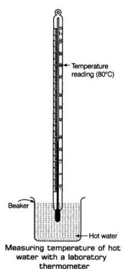
Note: To measure the human body temperature a laboratory thermometer cannot be used because as soon as we take out the bulb of the laboratory thermometer from the mouth of a patient, the mercury level wilt starts falling quickly (due to cooling of its bulb by air). So, this will provide a wrong value of the body temperature.
